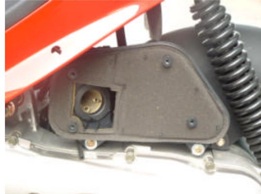
If there is too much accumulation of dust inside the air cleaner, it will reduce the output of engine performance and cause abnormal consumption of fuel.
